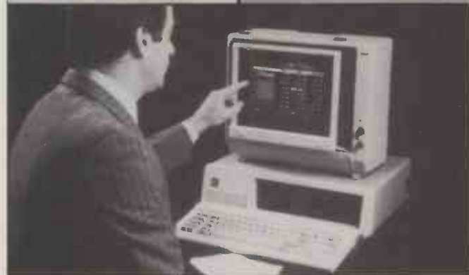
Top: The radical Maltron keyboard. Middle left: Tecmar's Escan. Middle right: Keytronic speech-recognition keyboard. Above: Ellinor's Touch Window screen fits in front of VDUs.
